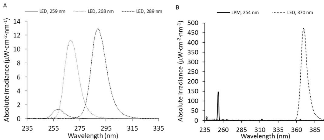
Fig. 1. Emission spectra of the (A) 259, 268, and 289 nm UV-LEDs and the (B) 253.7 nm LPM lamp and the 370 nm UV-LED in terms of absolute spectral irradiance.
