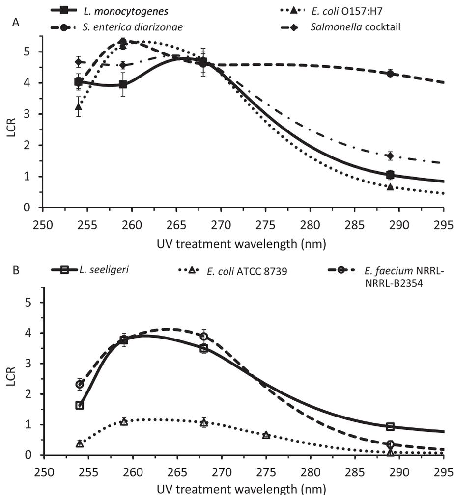
Fig. 3. The UV action spectra of *L. monocytogenes*, *E. coli* O157:H7, and *S. enterica diarizonae* (A); *L. seeligeri*, *E. coli* ATCC 8739, and *E. faecium* NRRL-B2354 (B) following UV treatment in saline suspensions at 253.7 nm using the LPM lamp, at 259, 268, 275, and 289 nm using UV-LEDs.
