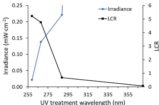
Fig. 5. Relationship between UV treatment wavelength, irradiance, and log count reduction of *E. coli* O157:H7 using UV-LEDs between 259 and 370 nm and a UV dose of 7 mJ·cm<sup>-2</sup>.
