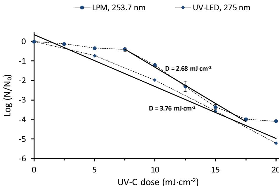
Fig. 2. Inactivation of *E. coli* ATCC 8739 in saline suspension when treated using an LPM lamp at 253.7 nm and UV-LED at 275 nm in comparison to previous results by Bowker, Sain, Shatalov, and Ducoste (2011) using *E. coli* ATCC 11229. Decimal reduction doses (D values) were calculated using the log-linear inactivation phase.
